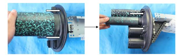
6.2.5 Inlet uncut cable and cut cable to inside of closure through oval and round ports.
