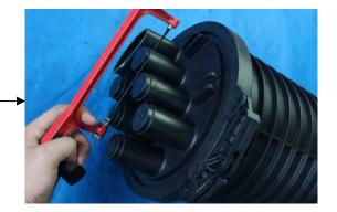
6.2.3 Rub and clean the inlet ports with a piece of abrasive paper to ensure the heat shrink and sealing performance.
