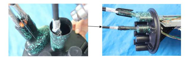
6.3.8 Insert the fibers into the buffering tube and lead into the cable storage plate and fasten with cable tie.
