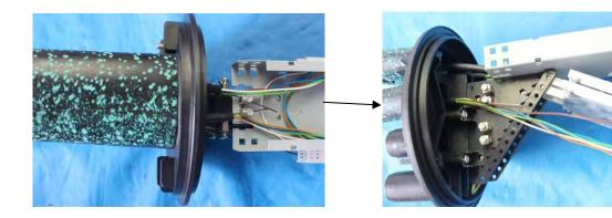
6.2.6 Wrap cable with foil paper properly to protect optical cable from heat and use the branching clip in the middle of cable and heat shrink tube.
