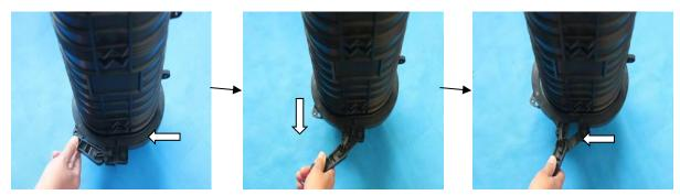
6.3.4 Release the screw of CSM fastener by special made key, insert uncut cable into heat shrink tube and oval port, position the optical cable in cable clamp and CSM in CSM fastener, then tight up the cable clamp for optical cable and CSM fastener for CSM
